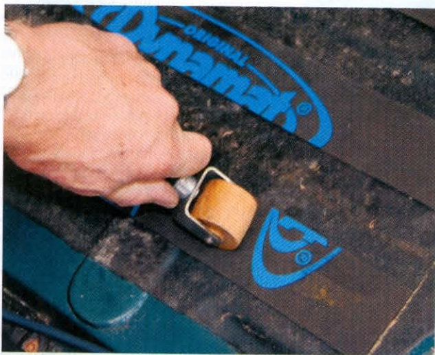
6 Use a roller to press the Dynamat strips in place, so they bond tightly with the sheetmetal.
