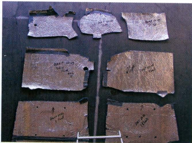
7 Quiet Ride precuts pieces of foil-backed Quality Heat Shield padding for the cowl, floor, roof, and trunk, so there's no custom fitting required in most cases.
